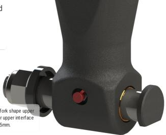
Formiko link FHL 02 is compatible with fork shape upper interface rotators. Designed for rotator upper interface width 80mm and rotator pin diameter 35mm.
