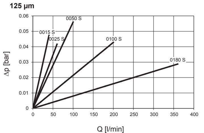
**3.2  $\Delta P$ -Q-GRAPHS FOR SUCTION FILTER ELEMENTS S.. FOR MOUNTING ON OUTSIDE OF TANK**
