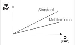
Thanks to its excellent cold start behaviour the Mobilemicron® element technology is used primarily in mobile applications but is also typically recommended for gear lubrication applications in systems with high temperature fluctuations and highviscosity oils (>ISO VG 100).
