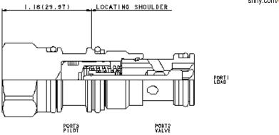
This valve is a pilot to open check valve. It has a non-sealed pilot, a steel seat, and is non-vented. It allows free flow from the valve (port 2) to the load (port 1) and blocks flow in the opposite direction. Pressure at the pilot (port 3) will open the valve from port 1 to port 2. Pilot pressure needed at port 3 to open the valve is directly proportional to the load pressure at port 1. Pressure at port 2 directly opposes pilot pressure.
