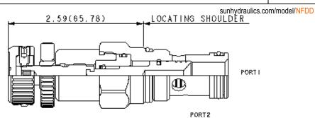
Needle valves are fully adjustable orifices used to regulate flow. They are infinitely adjustable from fully closed up to the maximum orifice diameter. They are not pressure compensated and may be used as flow controls or as shutoff valves.
