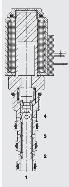
When the solenoid coil is de-energised, the valve allows flow in both directions between ports 3 and 2 and in both directions between ports 4 and 1. When the solenoid coil is energized, there is free flow through the valve in both directions between ports 3 and 4 and also between ports 1 and 2.
