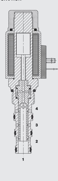
When de-energized, the valve allows flow from port 3 to 4 or from 4 to 3 and from port 1 to 2 or 2 to 1.
