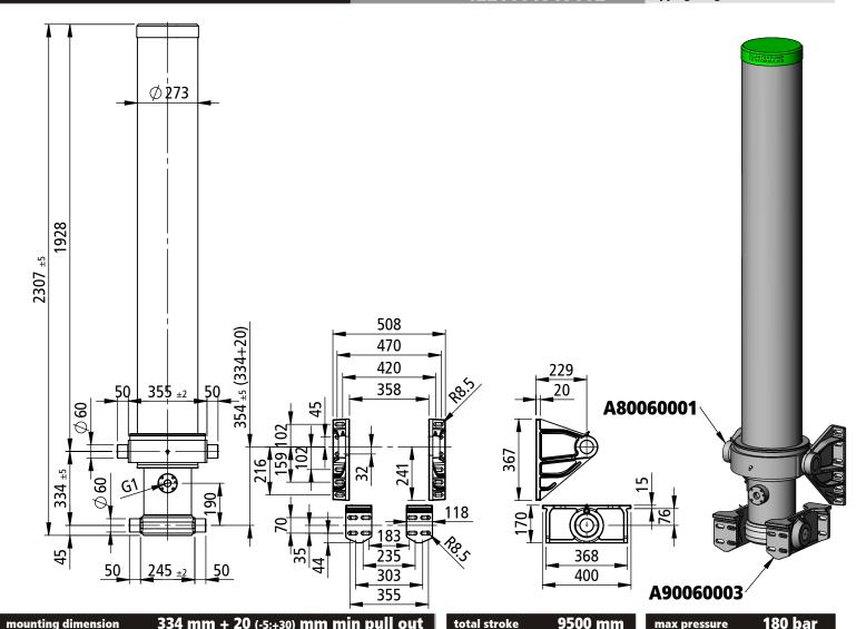
334 mm + 20 (-5;+30) mm min pull out 9500 mm total stroke max pressure 07082840 model: HFC 9500 191 5 CRN code: 4221601915002 weight: 533 kg extension number of stages: 5 2 4 5 191 169 149 129 111 diameter [mm] ------1890 1895 1900 1910 1905 stroke [mm] ---total: 9500 mm thrust [kN] at pmax 516 404 314 235 174 -----oil [dm³] 54.1 42.5 33.1 24.9 18.5 total: 173.1 dm<sup>3</sup>
